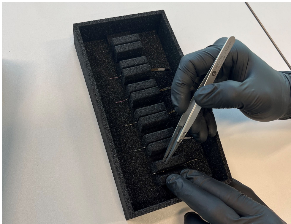
Figure 43: Removing the probe from the foam.
