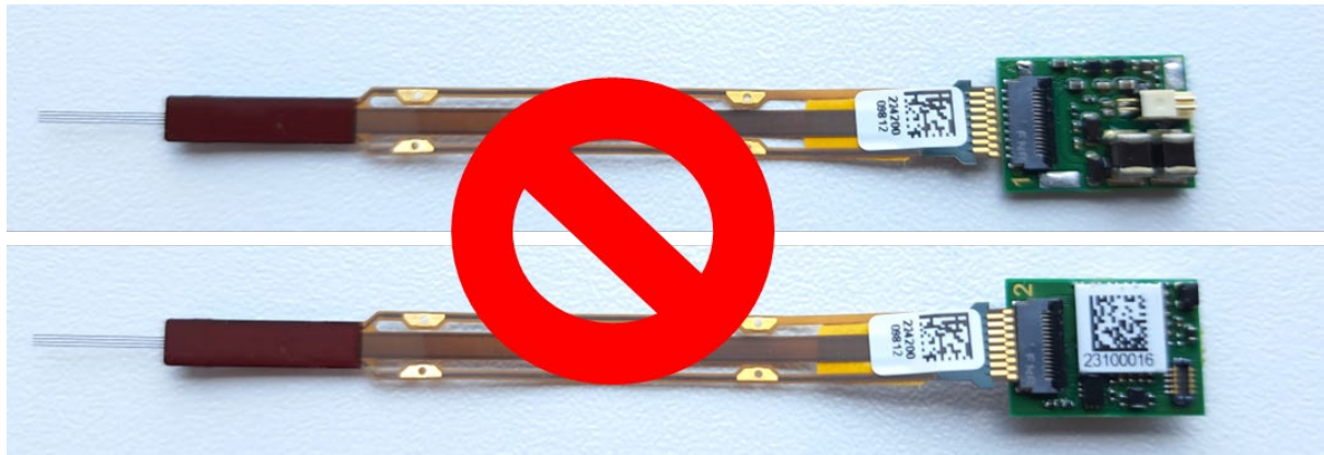
Figure 34: Wrong way to plug the flex in the ZIF connector. Top: front side dock, Bottom: back side dock.
