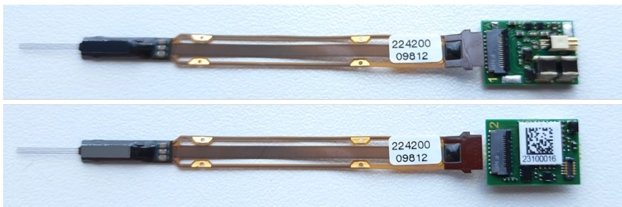
Figure 33: Correct way to plug the flex in the ZIF connector. Top: front side dock, Bottom: back side dock
