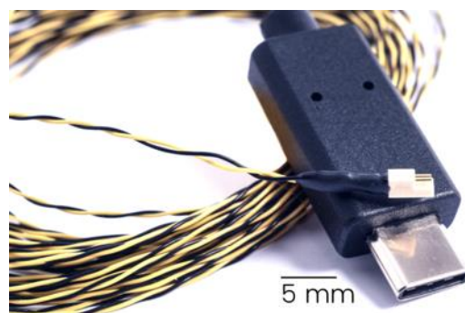
Figure 8: Twisted-pair interface cable with Omnetics-to-USB-C termination
