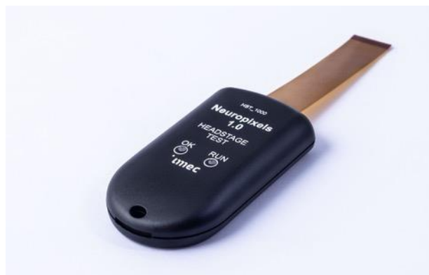
Figure 10: Headstage test dongle with flex cable that plugs into the ZIF connector of a headstage.
