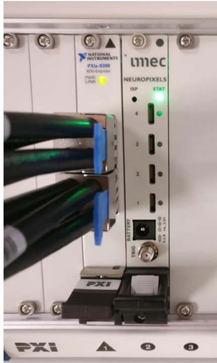
Figure 17: Global status LED of the PXIe acquisition module switching from red to green after correct installation.
