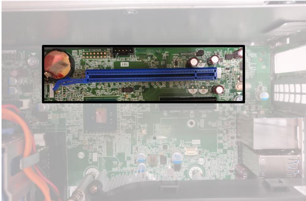
Figure 15: PCIe x16 slot on the PC motherboard.
